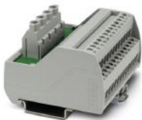
VARIOFACE module, with two equipotential busbars (P1, P2) for potential distribution, for mounting on NS 35 rails. Module width: 70.4 mm
